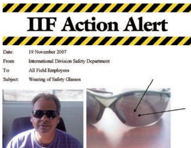
On Sunday 18 November 2007, Jon Soderberg, the Stores Manager was observing the placing of two pump liners on top of each other in the Yard. He was about 20 ft away from the operation. As the one liner was lifted by the forklift, a piece of metal broke free and struck Jon's safety glasses causing two hard impacts which cracked the left lens. Jon reported the incident to the office. His words were "NOW I KNOW WHY THE COMPANY HAS A 100% EYE WEAR POLICY" Thanks Jon for reporting the incident to us. This is the kind of incident that could have serious implications for any person not wearing their Personal Protective Equipment.
